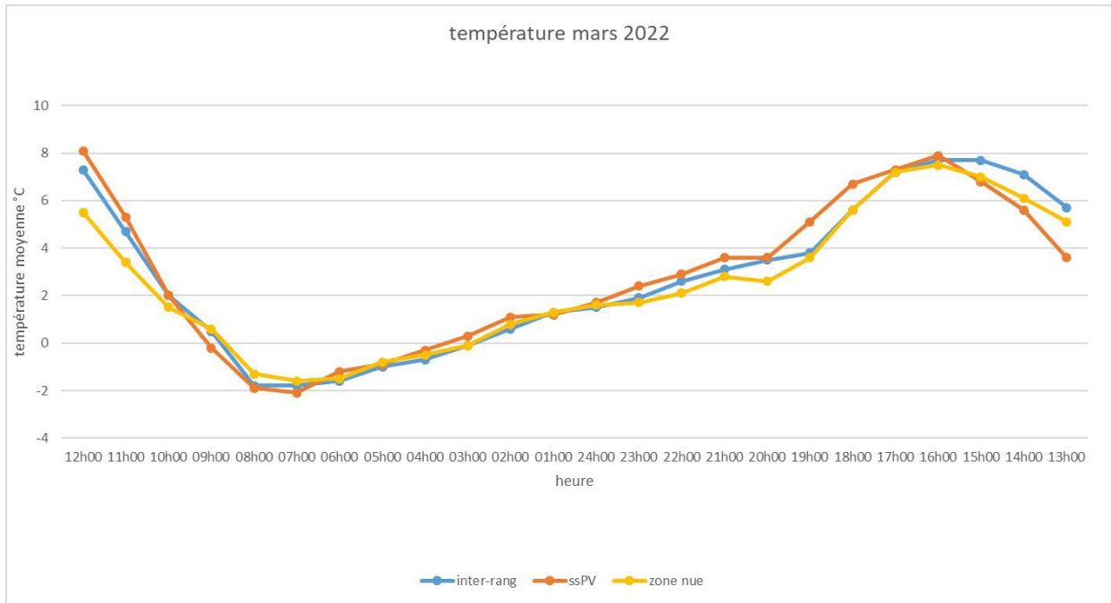
Average hourly temperatures over the 10th days of March 2022 (Note : The data recorded at the 2 stations in inter-row, not being significantly different, were averaged.)
